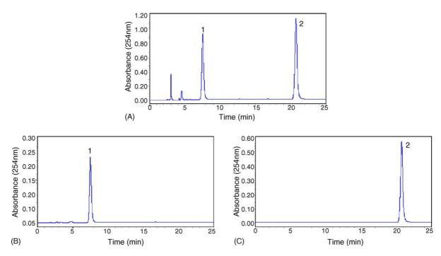
Fig. 2. HPLC chromatograms of the crude extract and the fractions obtained by HSCCC. Column: reversed-phase Lichrospher  $C_{18}$  (6.0 mm  $\times$  150 mm i.d. 5  $\mu$ m); mobile phase: CH<sub>3</sub>CN-H<sub>2</sub>O-HAC (25:75:1, v/v/v); flow rate: 1.0 ml/min; UV wavelength: 254 nm; (A) crude extract; (B) fraction "I" obtained by HSCCC; (C) fraction "II" obtained by HSCCC; peak 1: clemastanin B; peak 2: indigoticoside A.
