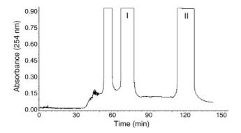
Fig. 3. Chromatogram of the crude extract by preparative HSCCC. Solvent system: ethyl acetate— $\underline{n}$ -butanol—water (2:7:9, v/v/v); stationary phase: upper phase; mobile phase: lower phase; flow rate: 2.0 ml/min; revolution speed: 800 rpm; separation temperature: 25 °C; sample size: 250 mg; sample loop: 20 ml; detection wavelength: 254 nm; retention of the stationary phase: 38.6%.
